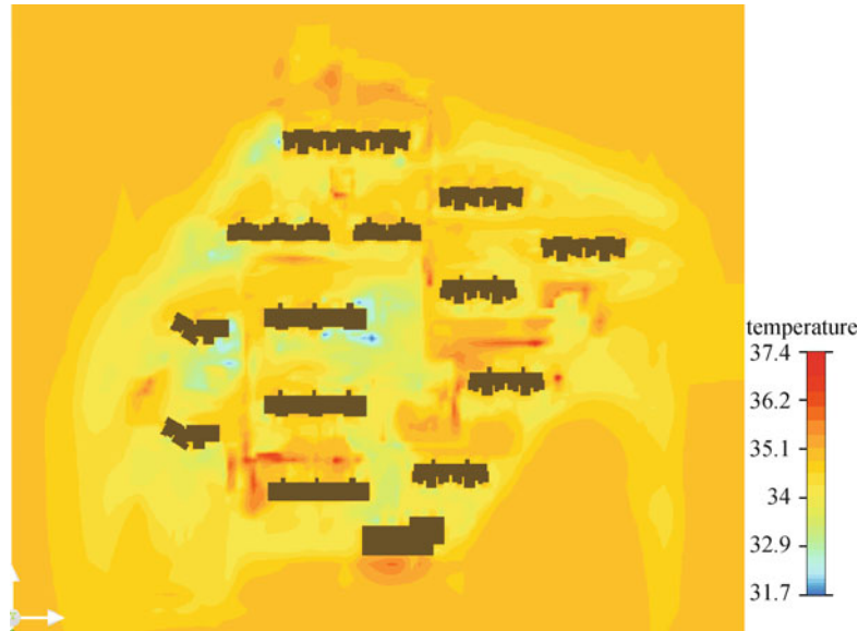
Fig. 8 Thermal performance analysis of a large residential area using CFD
